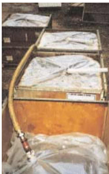
Fig. 3. Three typical IBCs in the background filled to within 5% of capacity with chimney apparatus attached, ready to start ferment, with a fourth IBC in the foreground being filled with must.
