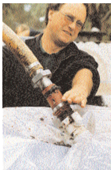
Fig. 2. Inventor/winemaker Andrew Hickinbotham releasing air from the bag via a simple air release point
